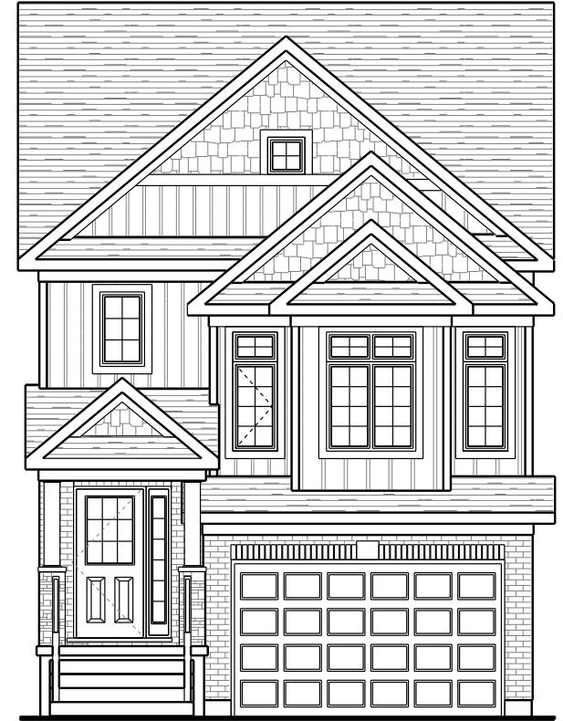
FRONT ELEVATION 'C' PN2204-3 1790 SQ. FT. (Includes 47 Sq. Ft. Open To Above)
